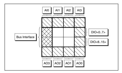
Figure 1-2. FPGA Logic Use in an Application with Many Fixed I/O Resources
